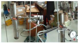
Figure 15: Sodium heat pipe with manometre
