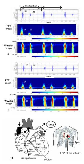
Fig.4: Audio-visual based recognition images analyzed for healthy heart sounds; a) at the apex and b) at the LSB of the 4th rib, c) an illustrative figure of the heart and the locations of auscultation.
