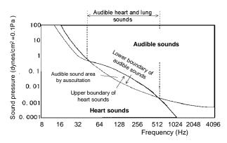
Fig.1: Diagram showing frequency bands of audible and heart sounds. Note that the audible sound area (40-600 Hz) by auscultation is small.
