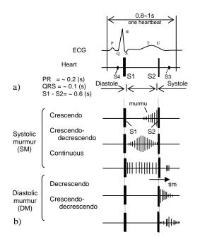
Fig.2: a) Relative timing of ECG graph and heart sounds at the apex and b) types of periodic murmur sounds (SM and DM), where S1, S2, S3, and S4 refer to the 1st, 2nd, 3rd, and 4th heart sounds, respectively (as seen in [10]).
