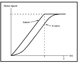
Figure 2: Available Ramp Shape in ACS800 drive – Linear and S-curve
