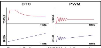
Figure 1: Performance of DTC Method Compared to Traditional PWM Method
