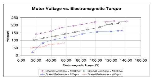
Figure 7: Motor Voltage vs. Electromagnetic Torque (Speed Control)
