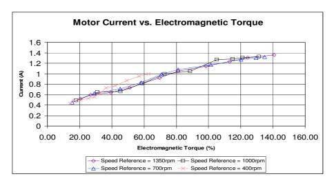
Figure 6: Motor Current vs. Electromagnetic Torque (Speed Control)
