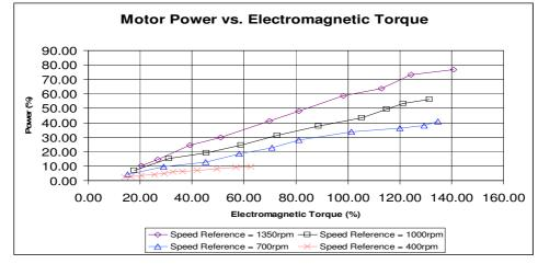
Figure 8: Motor Power vs. Electromagnetic Torque (Speed Control)
