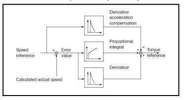
Figure 4: Block Diagram of the Speed Controller
