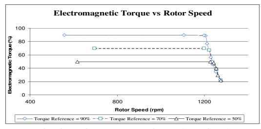
Figure 9: Rotor Speed vs. Electromagnetic Torque (Torque Control)
