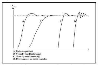
Figure 3: Speed Responses at a Speed Reference Step
